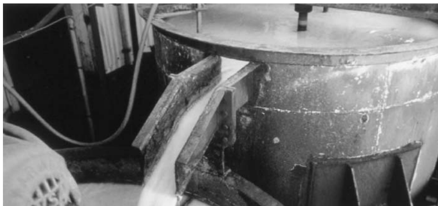
Figure 16.4 Ammonium diuranate (yellowcake) after solvent extraction. (Photo courtesy of UIC.) (Figure also appears in color figure section.)
